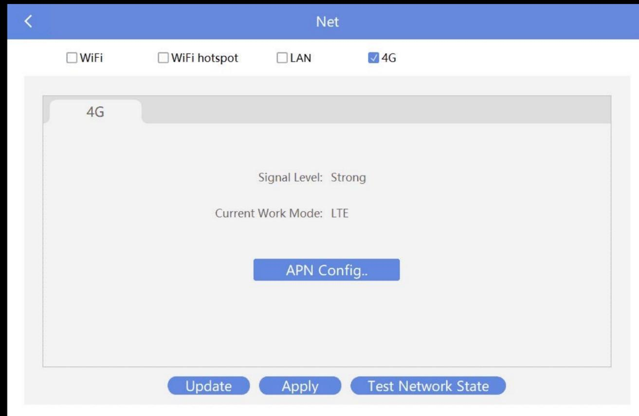
This for the 4G mobile solution if you use the 4G module with separate SIM-Card (PIN-FREE) with the 4G Antenna.
