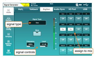
• Touch the 'Signal Type' value to select a type of signal.
