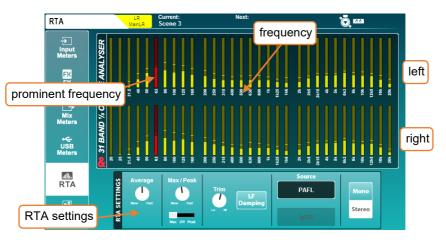
By default, the Meters screen '**RTA Souce**' is set to '**PAFL**' to match what is being sent to the headphone output and 12 segment LED meter. The source can also be switched to a specific fixed channel if desired.
