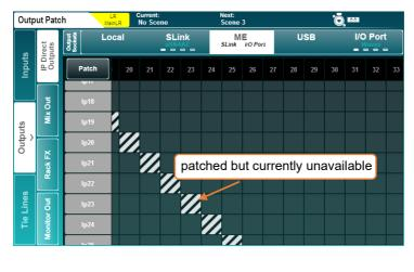
() All patching to a currently disconnected device will become active once the device is connected.
