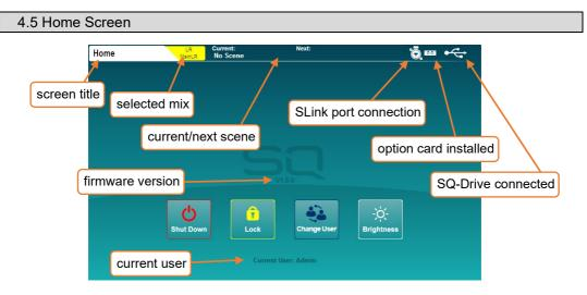
This is the first screen shown when powering on the SQ. It is also shown when no channels are selected, and '**Processing**' or '**Routing**' screen keys are active.
