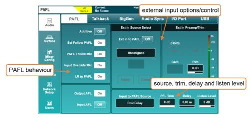
• Touch any button on the left of the screen to turn an option on or off.
