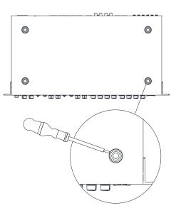
3. Install within the 19" rack making sure the unit is secure.
