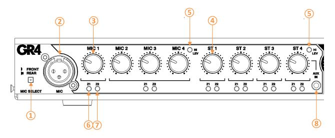
(1) MIC SELECT – a user selectable switch for MIC 1 input. MIC 1 signal can either be derived from the rear mount Euroblock or front mount XLR connectors. Use pointed object to select switch.
