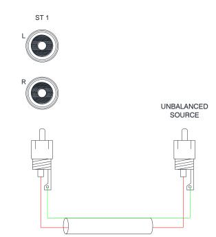
Unbalanced line input wiring example.
