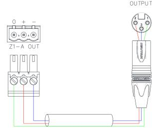
Balanced line output (XLR) wiring example.
