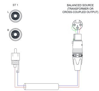
Balanced to Unbalanced input wiring example.
