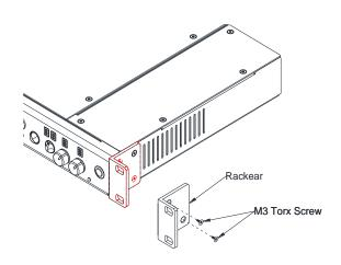
Be sure to use the supplied screws or exact replacements (damage to internal PCB's can result when using longer screws). 2. Using the small flat bladed screwdriver gently remove the four rubberized feet on the base of the unit.
