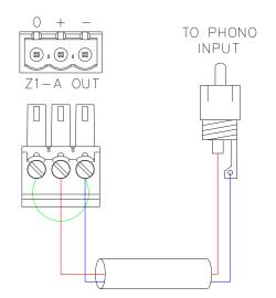
Balanced line output (Phono) wiring example.
