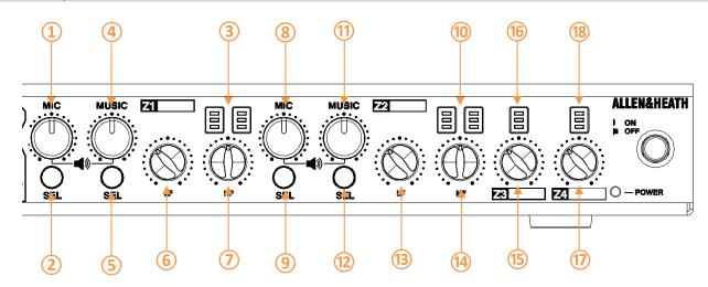
**1Z1 MIC MIX OUTPUT LEVEL** – Adjustable rotary level control for MIC Mix to Zone 1. Output level control Off to +6dB.
