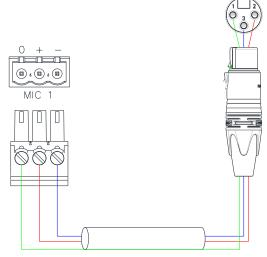
Balanced microphone input wiring example.
