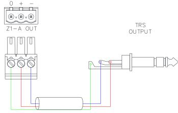
Balanced line output (TRS) wiring example.
