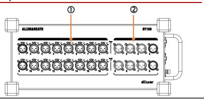
① Input sockets Balanced XLR mic/line inputs with +48V Phantom Power indicator. The preamps are built into the DT168 and their Gain, Pad and +48V are controlled from the network.
