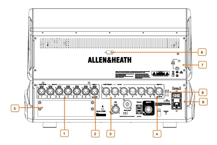
Mic/Line inputs – 6x recallable preamps for balanced or unbalanced microphone and line level signals. Gain, Pad and 48V are digitally controlled within the preamp.
