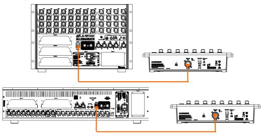
Power up the IP8 by plugging the external PSU into the DC In socket. The port Lnk/Err indicator flashes at a steady rate when the link is established. The unit Name and IP address are displayed on the LCD Displays for easy identification of the unit. After a few seconds the IP8 will display the assignments and functions if any have been set for the unit.
