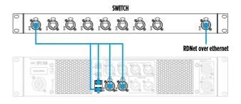
Connecting 2 different ports of the device to the external switch a full redundancy is achieved.
