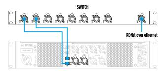
Each XPS 16K device must be connected to a different switch port.
