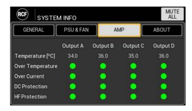
Shows the status of device power amplifiers modules for each output, as well as the protections operativity.
