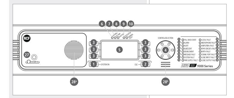
**SYSTEM ON** button: press and hold to turn amplifier on (when off). This button also works as fault acknowledge: press it to remove the displayed fault indication.
