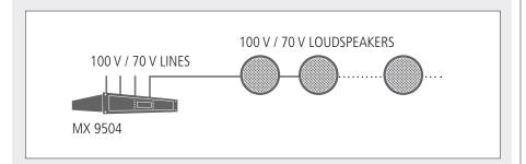
A system that requires a higher output power or a larger number of zones can be obtained by adding one or more system amplifiers model UP 9501 (1 x 500 W), UP 9502 (2 x 250 W) or UP 9504 (4 x 125 W) to the MX 9502 / MX 9504, connected through the dedicated RCF FLEXCOM data-link port.
