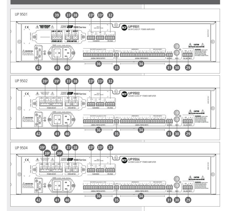
**29 FALL BACK INPUT:** monitored audio input (balanced, 'line' level, for removable connector) to be used for emergency announcements. This input can be used even in case of software crash.
